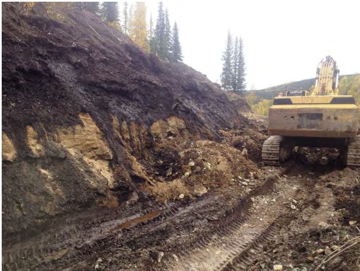
FIGURE 13: SIDEHILL BEDROCK AND OVERLYING GRAVEL ON CLAIM NO. 2 BELOW DURING THE 2014 SEASON
