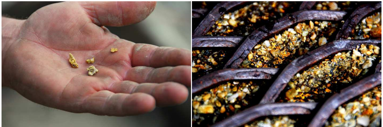
FIGURE 15: EXAMPLES OF GOLD RECOVERED ON JUNE 10, 2014 AFTER 6 HOURS OPERATION AT 60 YARDS PER HOUR
